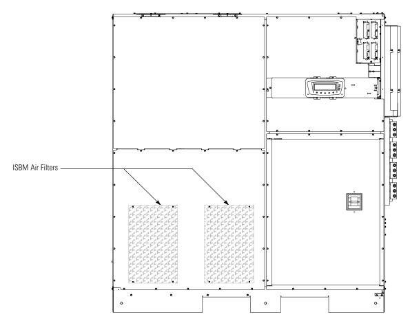
Figure 9-1. ISBM Section Air Filter Locations
